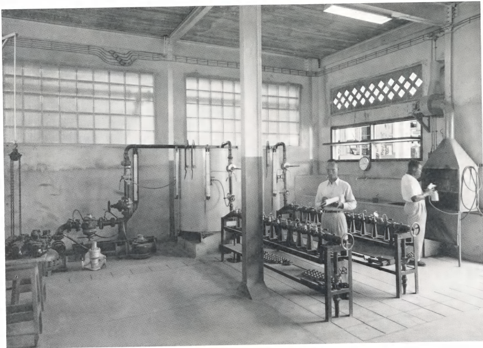
METER-HERSTELINRICHTING TE MUNDO-NOBO LUGA PA DRECHAMENTU DI METER NA MUNDO-NOBO PLACE TO REPAIR WATERMETERS AT MUNDO-NOBO
